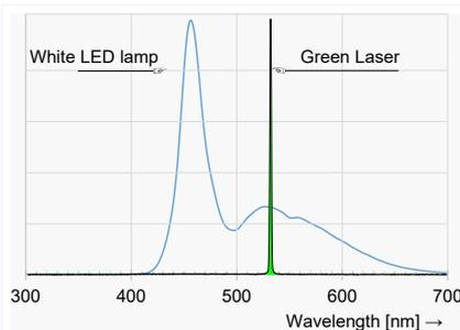
Fig. 4.44: Spectral distribution of the used light sources
