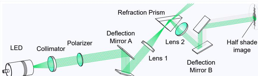
**Fig. 2.36: Refractometer setup**
