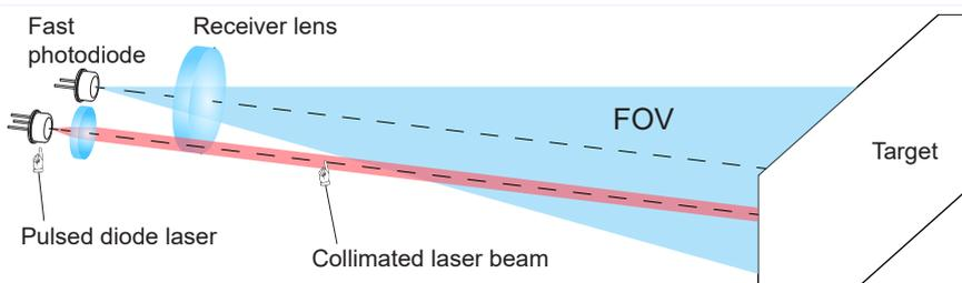
The emission of the pulsed diode laser is collimated to an almost parallel laser beam. At a certain distance it hits the target from which scattered light travels back depending on the scatter properties of the target. The receiver lens captures according to its field of view (FOV) a small fraction of it and focuses it onto a fast photodiode. Due to the fact that only a small fraction of the incident light comes back, a fast and sensitive amplifier is needed.
