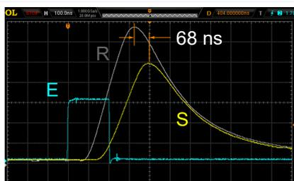
Fig. 2.28: Measurement of the time of flight
