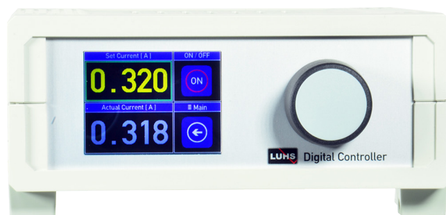
Fig. 15: DC-0270 Filament and LED controller
