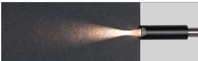
Fig. 22: The light output from the fiber bundle included with the OSL2 lamp. It show the beam when the focusing packages is attached.
