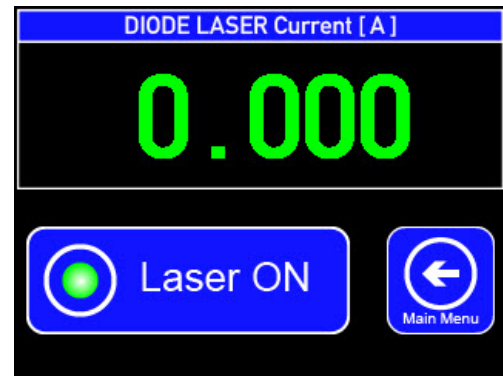
Fig. 44: Injection current settings
