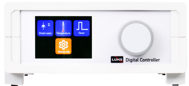
Fig. 39: Front view of the diode laser controller and timer
