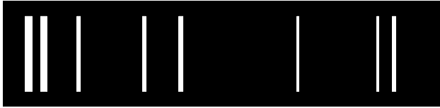
Fig. 7: Photograph of the emission of a light source with the corresponding energy level showing a commonly known line spectrum.
