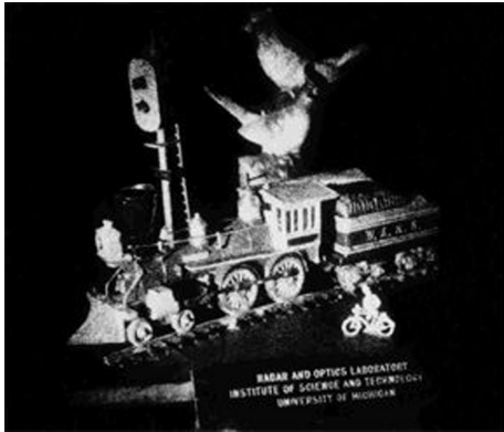
Fig. 1: Emmett Leith and Juris Upatnieks (MSE EE '65) displayed their revolutionary laser transmission hologram of a toy train at the Optical Society's 1964 Spring Conference
