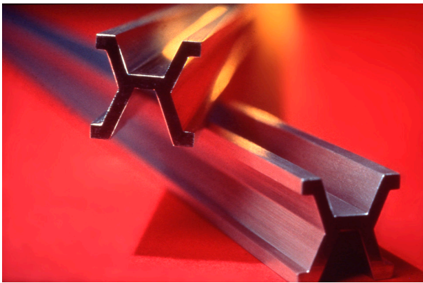
Fig. 1: Definition of the metre by a platinum-iridium bar
