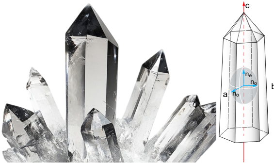
Fig. 7: Natural grown quartz crystal (left) and its exact structure (right).
