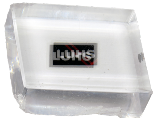
Fig. 5: The image above shows the double refraction of a calcite crystal.
