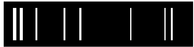
Fig. 6: Recording the emission of a light source with corresponding energy levels results in a line spectrum
