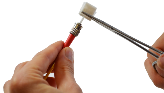
Fig. 13: Cleaning the front face of an optical fibre
