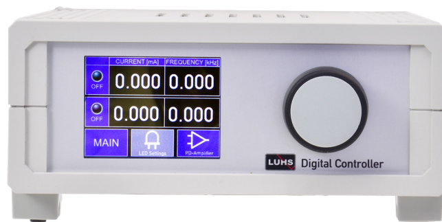
Fig. 19: DC-0030 Dual channel LED transmitter
