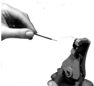
Fig. 27: Removing the protective plastic cover with the provided tool
