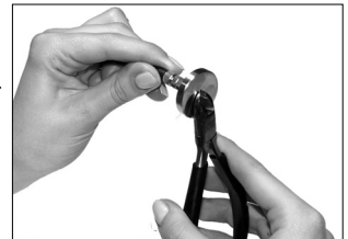
Fig. 28: Shortening of the out standing bare fibre
