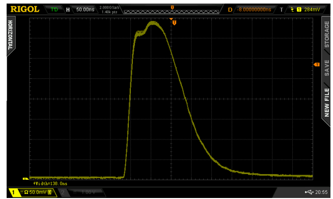
Fig. 24: Light pulse, settings 150 ns, 20V
