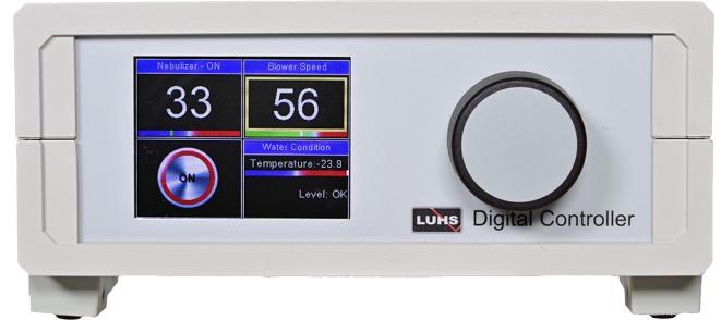
Fig. 26: Front view of the US Particle Generator Controller
