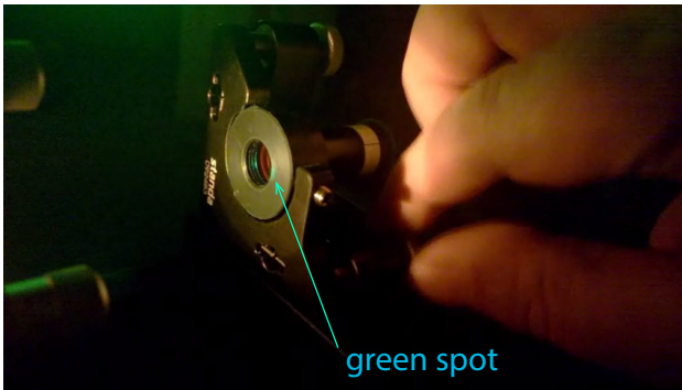
Fig. 46: Aligning the green spot viewing through the GG495 filter
