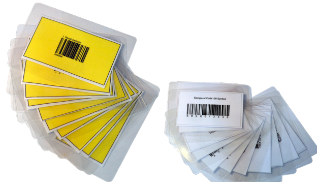
Fig. 44: Set of configuration bar code symbol cards (left) and sample bar codes
