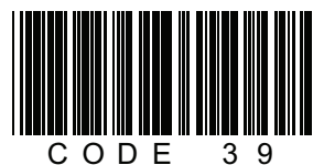
Fig. 11: Code 39 Symbol with the Information ‘‘CODE 39’’
