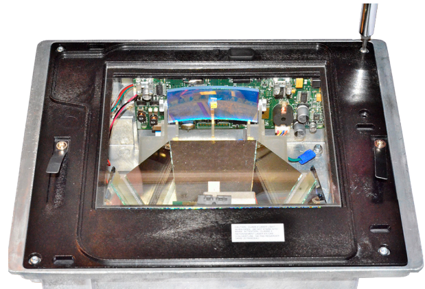
Fig. 49: Remove the screw of each corner
