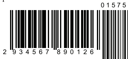
Fig. 9: EAN 13 Symbol with EAN 5 Add On
