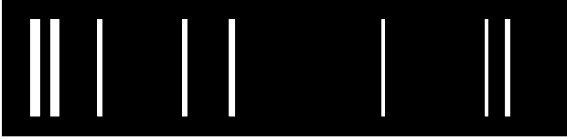
Fig. 18: Photograph of the emission of a light source with the corresponding energy level showing a so-called line spectrum.
