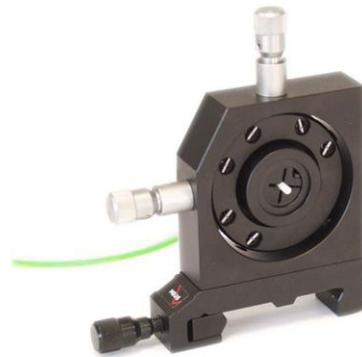
**Fig. 25: Module O regulatory fibre holder**
