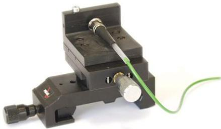
**Fig. 24: Module N Fibre holder on translation stage**
